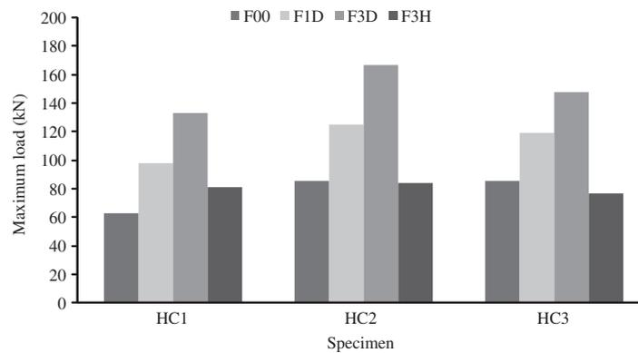
Figure 5 Maximum loads vs. strengthening configurations for  $a/d=0.40$ .
