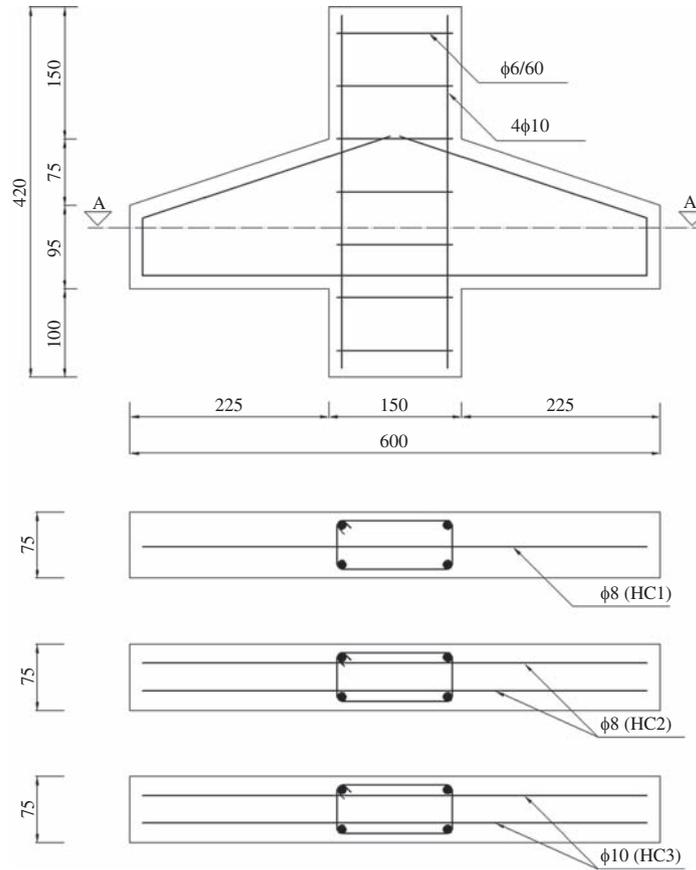
**Figure 1** Reinforcement detail of corbel specimens (units are mm).
