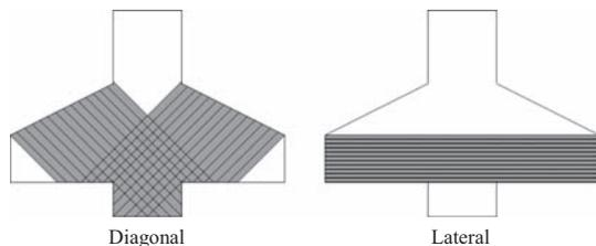
**Figure 2** GFRP wrapping configurations.
