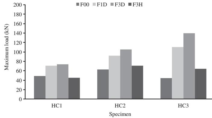
Figure 6 Maximum loads vs. strengthening configurations for  $a/d=0.80$ .
