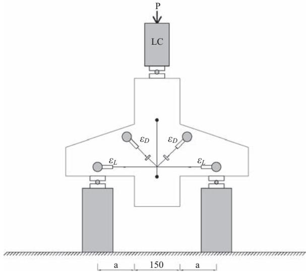
**Figure 3** Loading set-up and deformation measuring device locations (units are mm).
