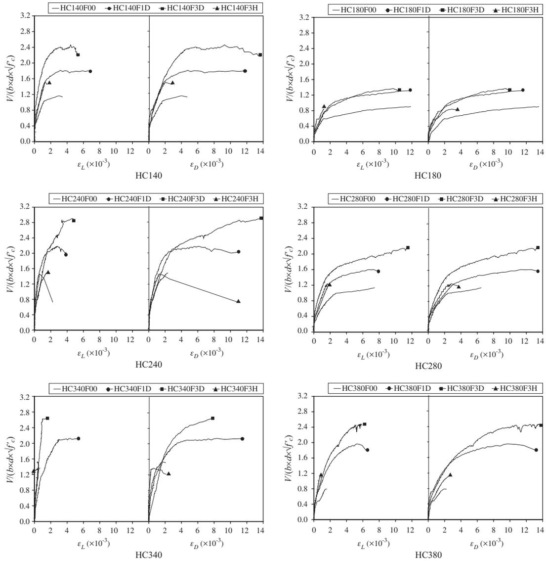
**Figure 8** Normalized shear stress vs. lateral ( $\epsilon_L$ ) and diagonal ( $\epsilon_D$ ) strains.
