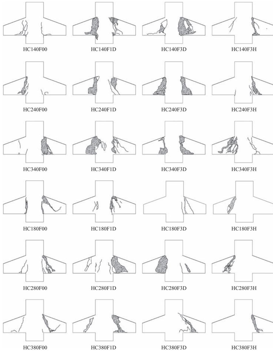
Figure 4 Crack pattern for corbel specimens.
