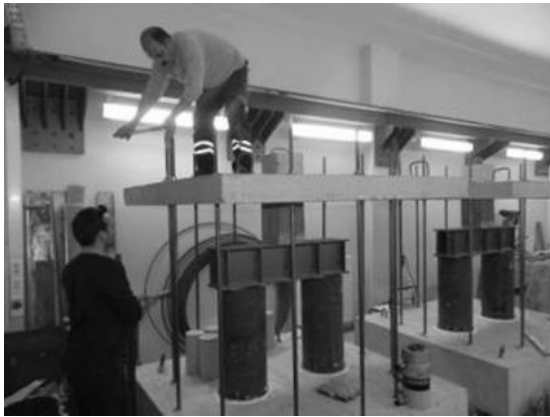
Fig. 2. General view of test setup and sustained load application
