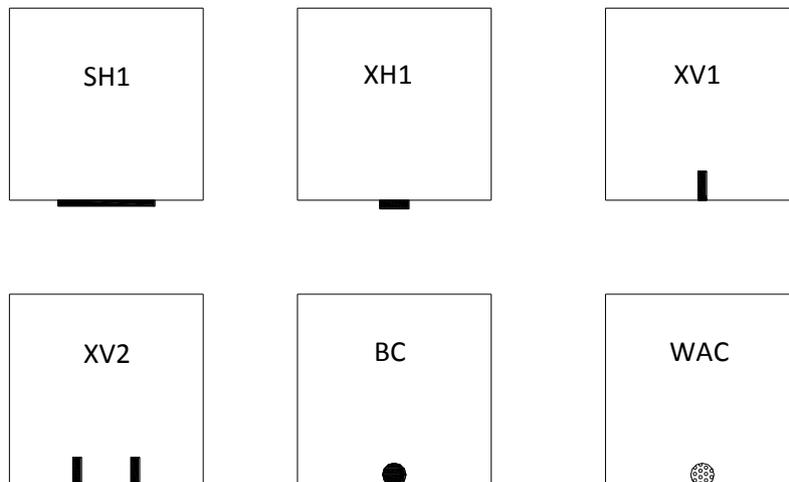
**Figure 2** - FRP strengthening schemes of the test specimens
