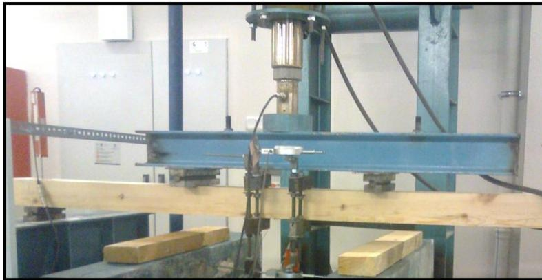
**Figure 3 - Test Setup**
