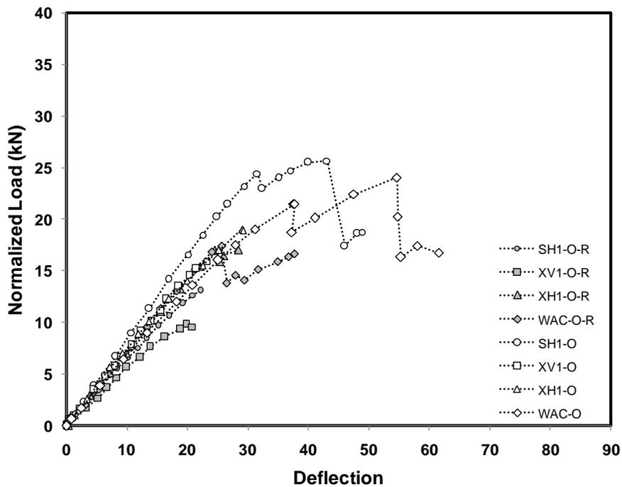
Figure 5 – Load-deflection response of Black Pine Specimens
