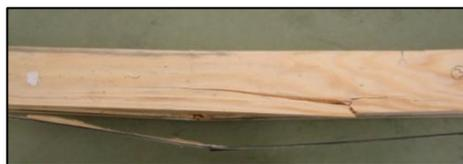
cross grain tension failure
