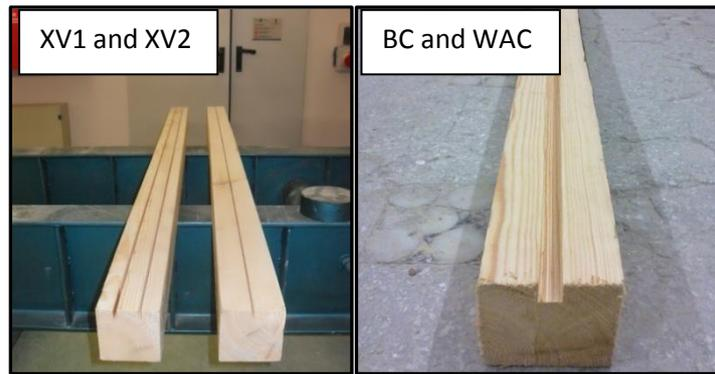
**Figure 1** - Grooves prepared for FRP installation
