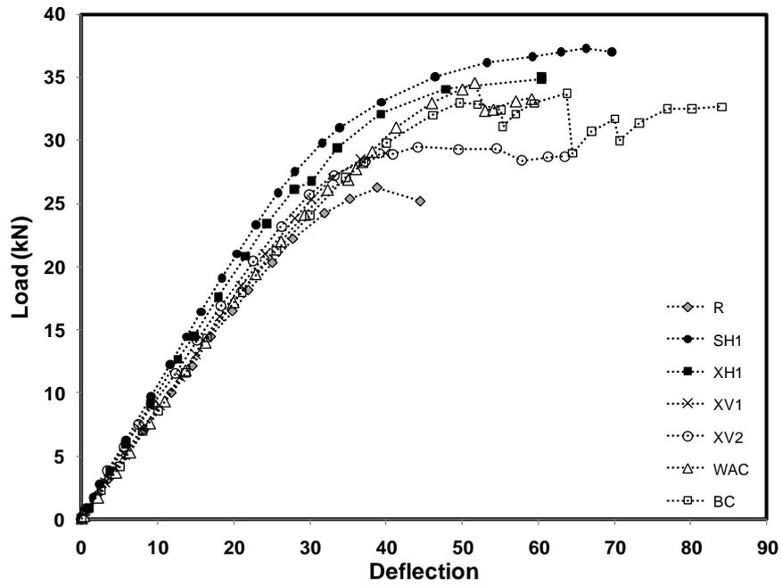
Figure 4 – Load-deflection response of Yellow Pine Specimens
