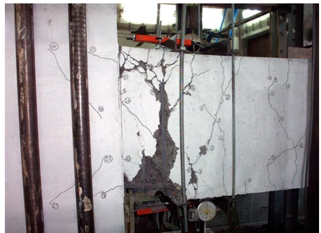
Fig. 8. Damage in monolithic specimen at 4% drift level.
